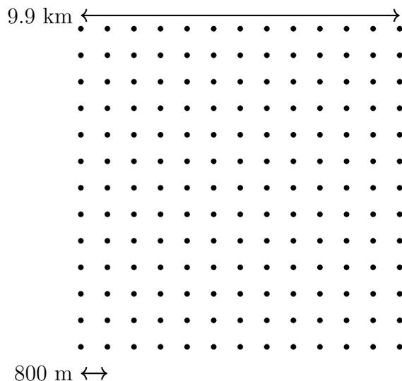
**Figure 3:** The field of 169 wind turbines (13x13).
