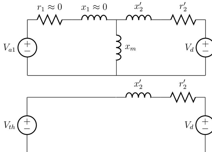
**Figure 1:** A circuit representing the turbine (top) and its reduced form (bottom).
