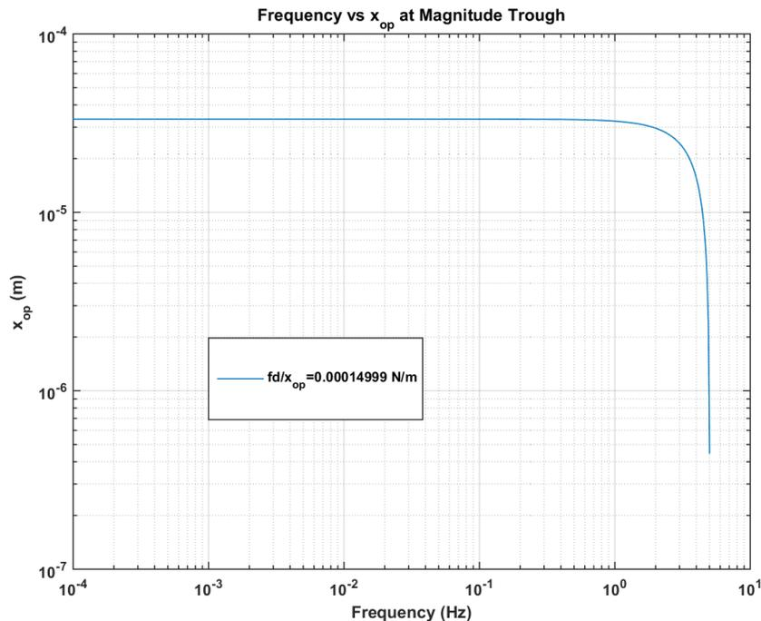
**Figure F.2:** A plot of Frequency vs Plate Position with the Dynamic Stiffness set to 0.00014999 N/m.
