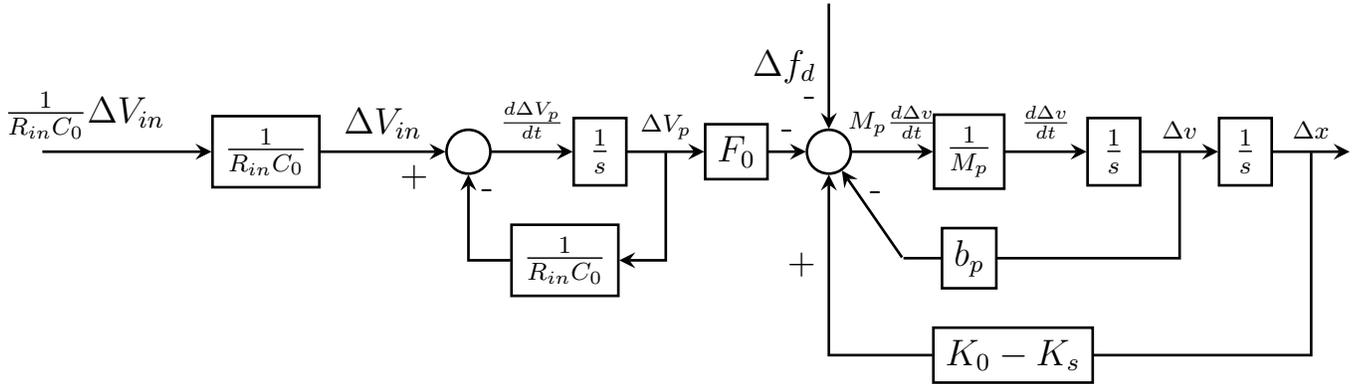
Figure 4.2: The Reduced Operating Point Model in block diagram form.
