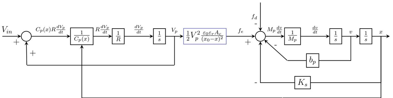
**Figure 2.1:** The state space model in block diagram form. It is important to note that the capacitance function is  $C_p(x) = \frac{\epsilon_0 \epsilon_r A_c}{x_0 - x}$ .
