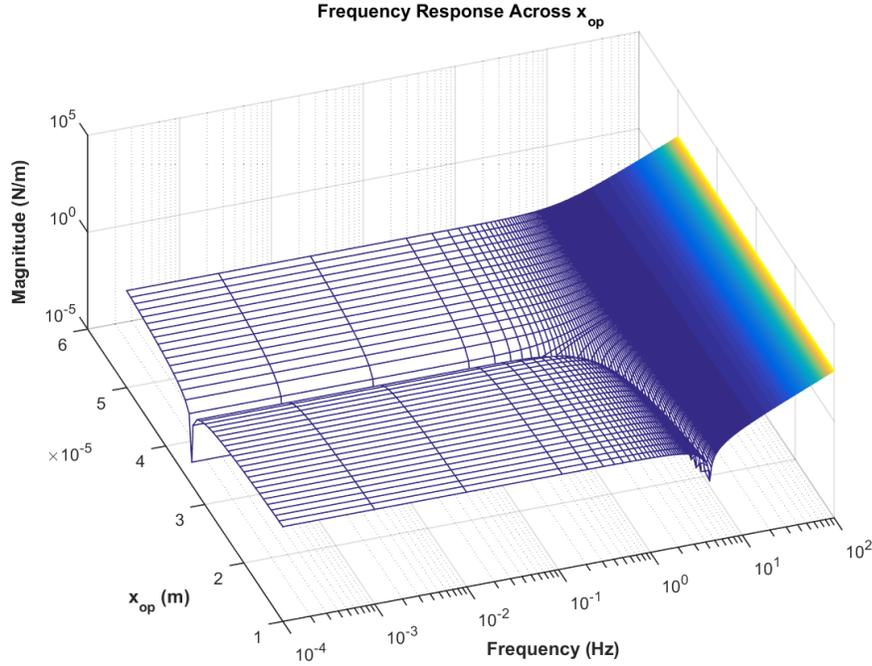
**Figure F.1:** A plot showing Frequency ( $f$ ) vs Plate Position ( $x_{op}$ ) vs Magnitude ( $\frac{\Delta f_d}{\Delta x}$ ) shows a better big picture of what is going on with the resonance frequency.
