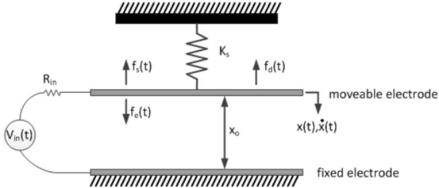
**Figure A.1:** A schematic diagram of the Digital Micromirror Device (DMD).
