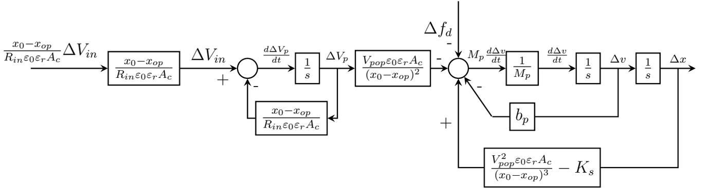
Figure 3.1: The Operating Point Model in block diagram form.
