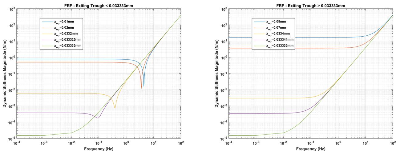
**Figure F.3:** As the operating point position  $x_{op}$  is varied near the trough, getting smaller than 0.033333mm (left) leads to resonant frequencies while getting larger than 0.033333mm (right) leads to no resonant frequencies.
