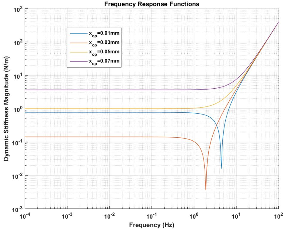
**Figure 6.1:** A plot of Dynamic Stiffness vs Frequency for four values of  $x_{op}$ .
