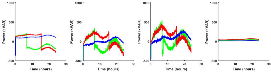
**Figure 9:** Reactive power plots for power just upline from capacitor banks. This is after CapBank0, CapBank1, and CapBank2 have been enabled.
