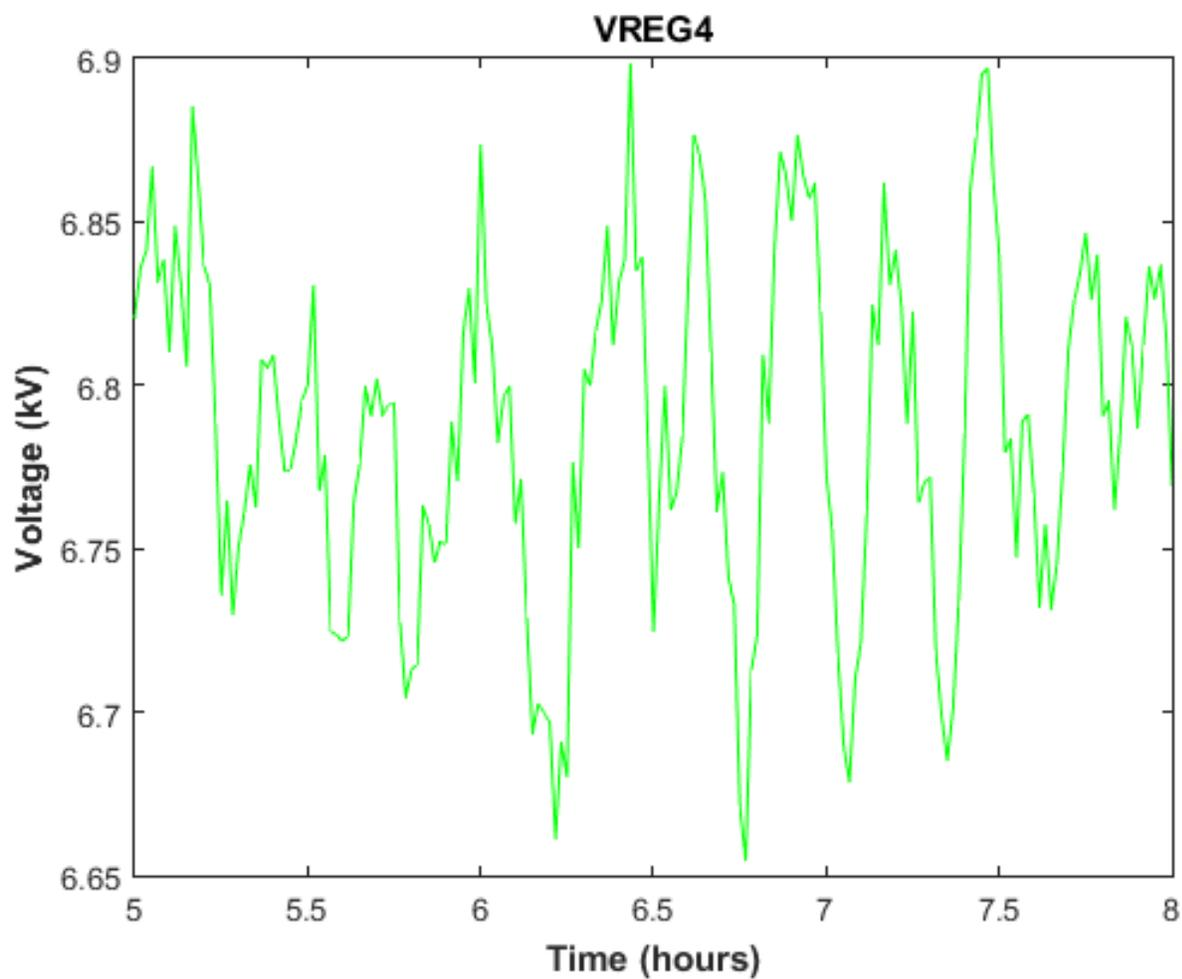
**Figure 3:** A zoomed in segment of VREG4's voltage during a January 11, 2014 simulation. The maximum peak to peak distance in this segment is 243V.
