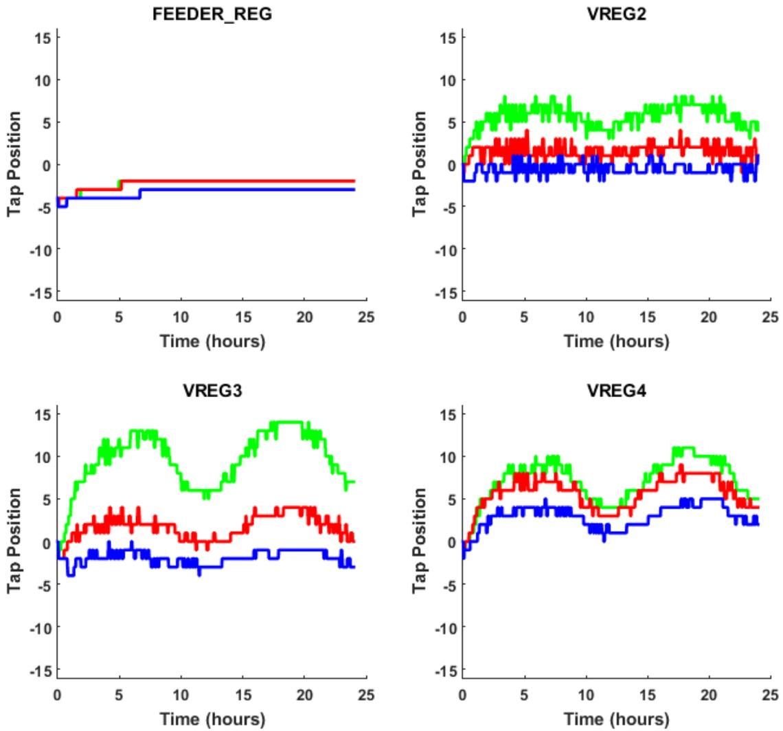
**Figure 1:** Plots showing regulator tap changes per phase for the winter day of January 11, 2014. Green is Phase A, Red is Phase B, and Blue is Phase C. Tap change totals per phase for these plots are shown in Table 1.
