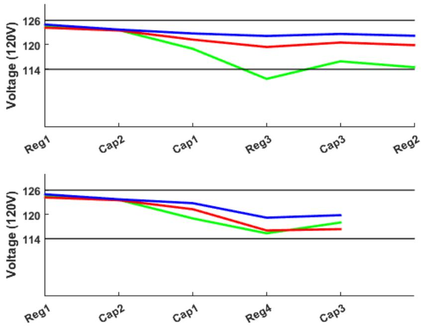
**Figure 12:** Voltage profile for the two legs of the feeder showing marked improvement of voltages.
