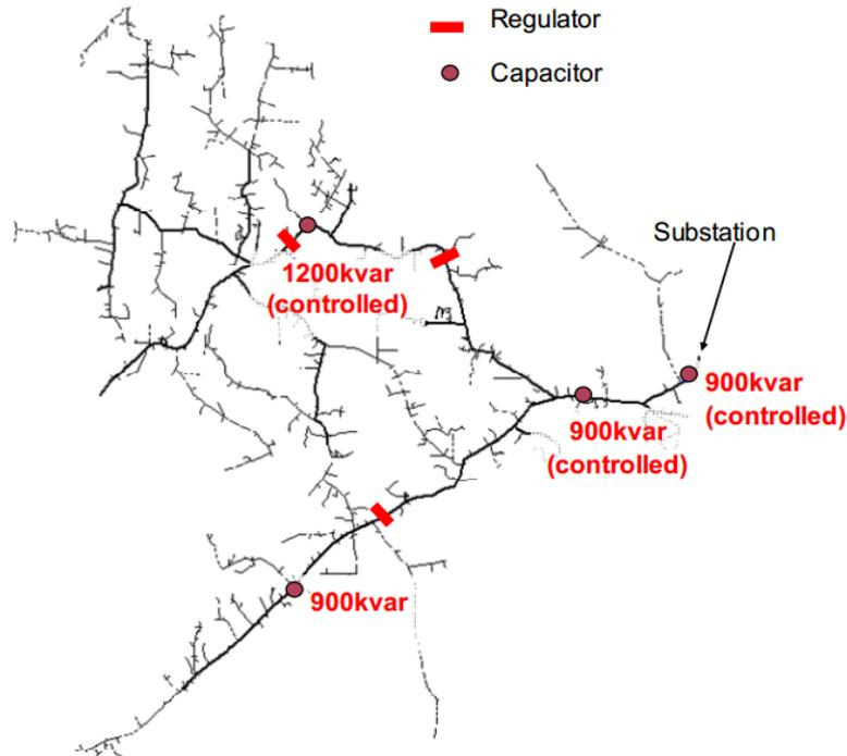
**Figure 4:** A one-line diagram of the IEEE 8500 Node Test Feeder circuit.[1]
