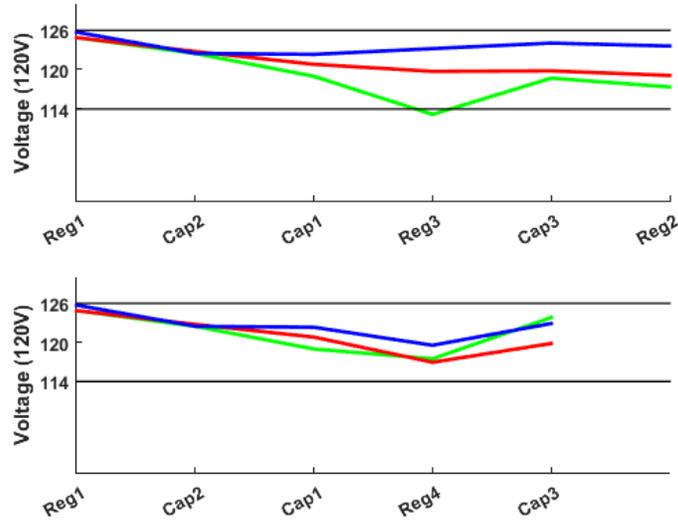
**Figure 2:** Initial voltage profile of the system showing voltage levels on to upper (top) and lower (bottom) legs of the feeder.
