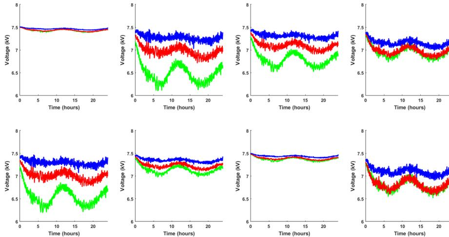
**Figure 6:** The voltages of each regulator and capacitor throughout the day. The top row of plots is voltage for the regulators in order, FEEDER.REG, VREG2, VREG3, VREG4 while the bottom row of plots is capacitors in order, CapBank0, CapBank1, CapBank2, CapBank3.
