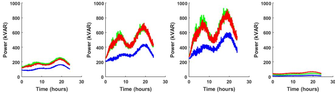
**Figure 8:** Reactive power plots for power just upline from capacitor banks, in order from left to right, for CapBank0, CapBank1, CapBank2, CapBank3.
