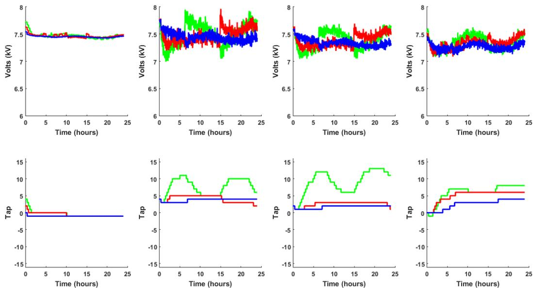
**Figure 11:** Voltages just upline from regulators and the tap changes that each regulator made in response to the voltage.
