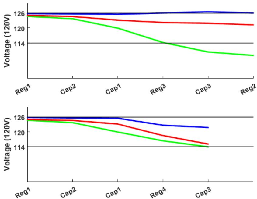
**Figure 10:** The voltage profile seen after CapBank0, CapBank1, and CapBank2 were enabled.
