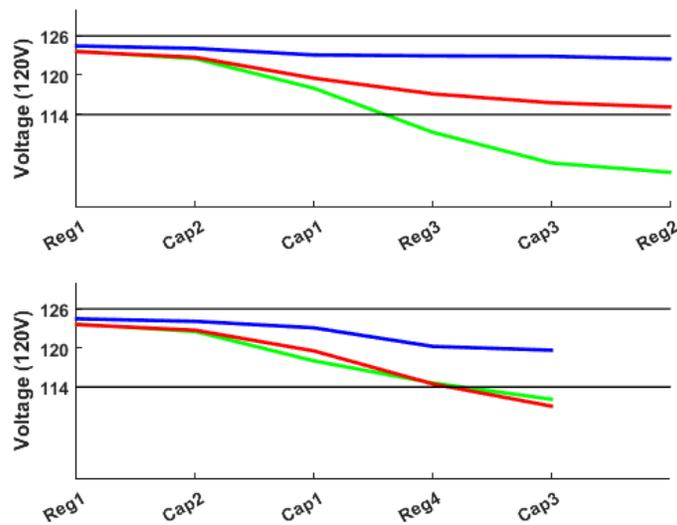
**Figure 7:** The voltage profile when all regulators and capacitors are turned off. There are two plots because the feeder splits into two legs.
