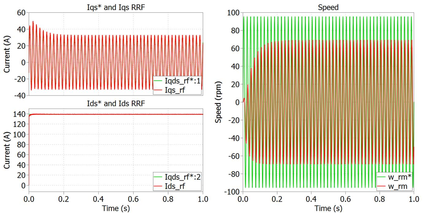
**Figure 17:** The current command (green) and response (red) for a 50 Hz sinusoidal speed command (left) and speed (right). The speed is being attenuated, as expected, since the frequency here is the same as the speed loop bandwidth.
