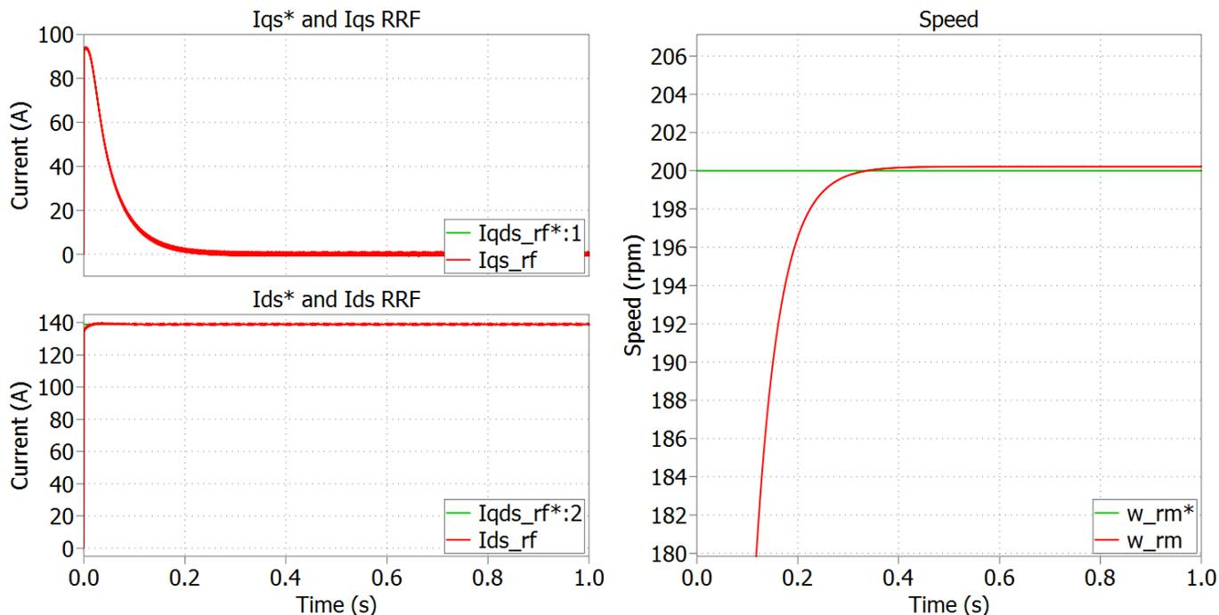
**Figure 15:** The current command (green) and response (red) for constant commanded speed input (left) and response speed (right).
