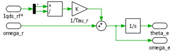
**Figure 9:** The Slip and Angle block from the simulation.
