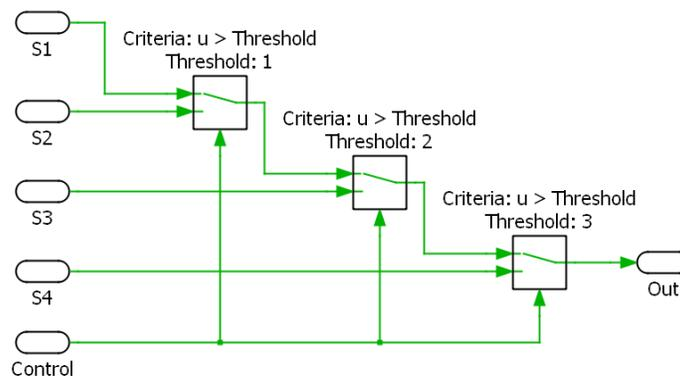
**Figure B.2:** The Switch block with controlled switches configured such that a 1 sends through S1, a 2 sends through S2, etc.
