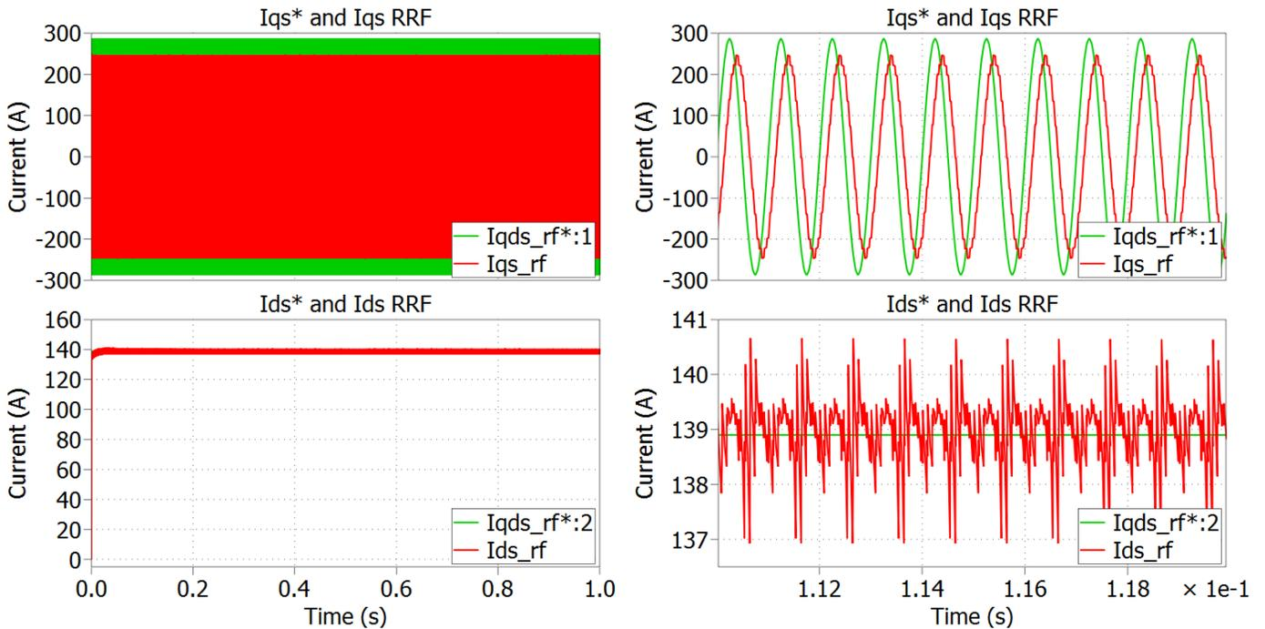
**Figure 14:** The current command (green) and response (red) for sinusoidal torque input at 1000 Hz. A full second is shown on the left and a few periods on the right. The response current is  $\frac{1}{\sqrt{2}}$  times the commanded current since the frequency is equal to the bandwidth.
