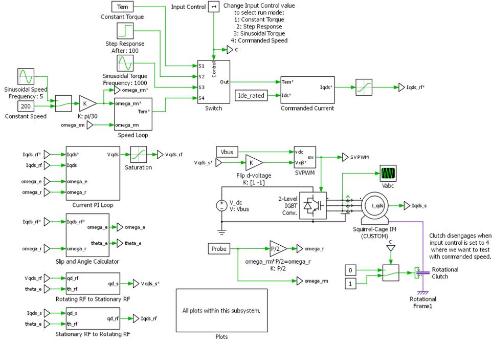
**Figure 1:** A top-level schematic of the TESLA IM simulation in PLECS. The various control scenarios can be seen in the upper-left region of this schematic.
