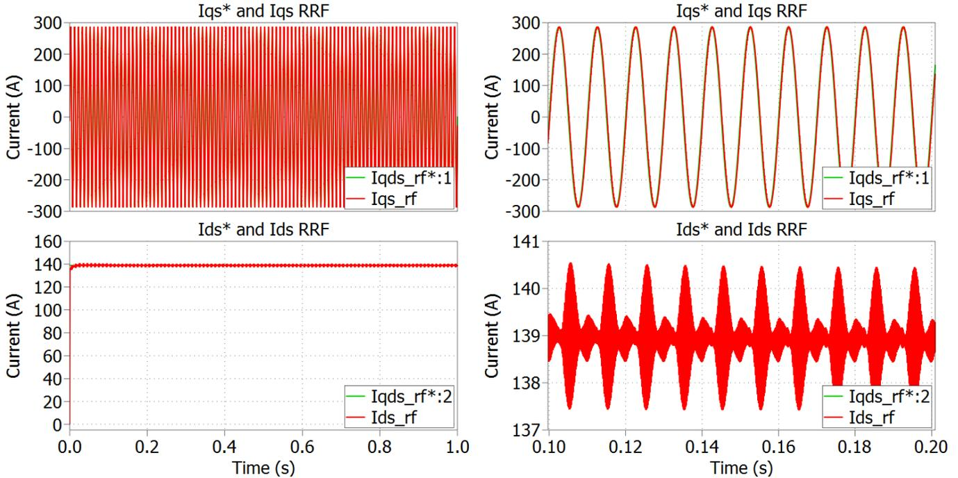
**Figure 13:** The current command (green) and response (red) for sinusoidal torque input at 100 Hz. A full second is shown on the left and a few periods on the right. The current ripple spans 2.2 Amps.
