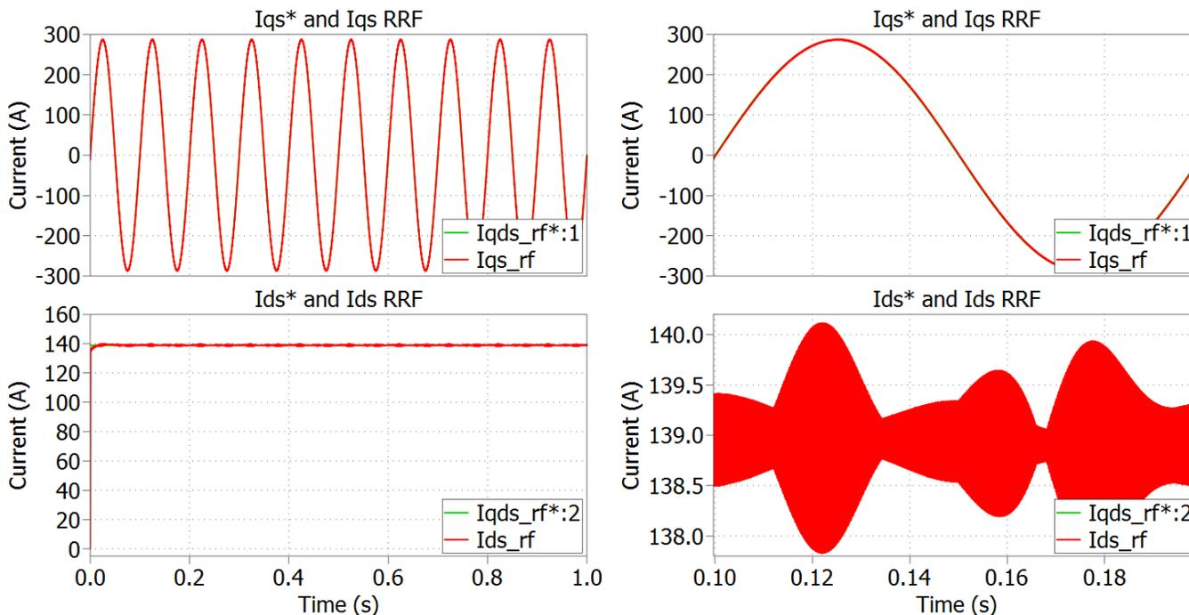
**Figure 12:** The current command (green) and response (red) for sinusoidal torque input at 10 Hz. A full second is shown on the left and a single period on the right. The current ripple spans 2.2 Amps.
