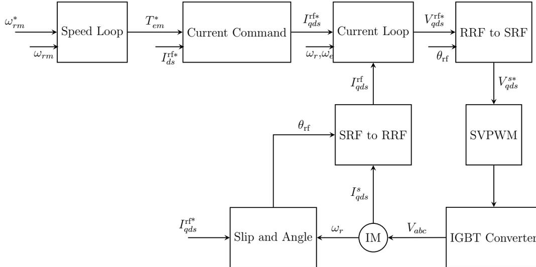
**Figure 2:** A simplified block diagram of the TESLA IM and the indirect field orientation control.
