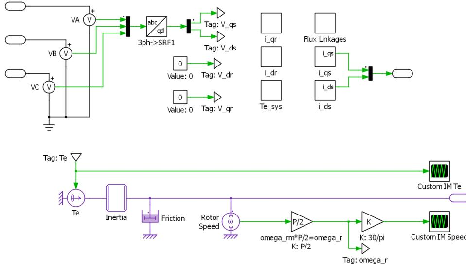
Figure 7: The schematic of the custom Squirrel-Cage IM.
