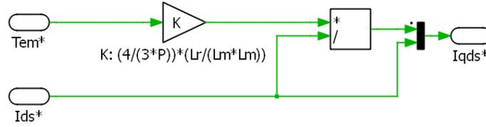
**Figure 4:** The Current Command block from the simulation.
