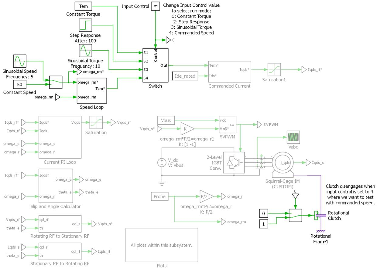
**Figure B.1:** The full system schematic from PLECS with the scenario control areas highlighted.
