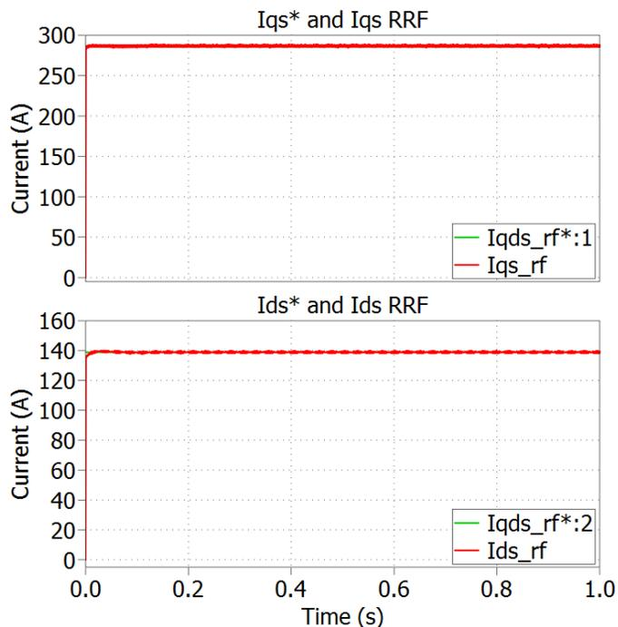
**Figure 10:** The current command (green) and response (red) for a constant commanded torque.
