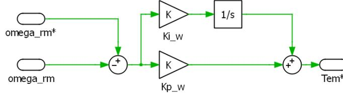
**Figure 3:** The Speed Loop block from the simulation.
