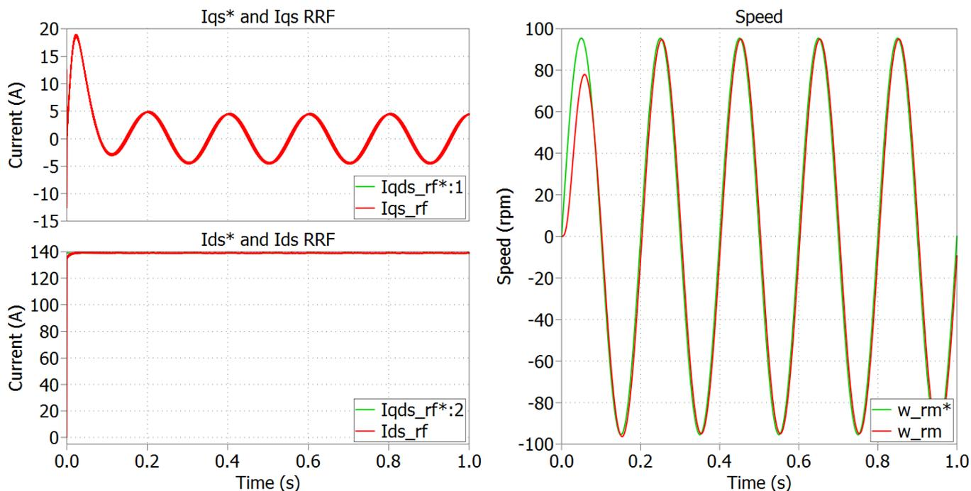
**Figure 16:** The current command (green) and response (red) for a 5 Hz sinusoidal speed command (left) and speed (right).
