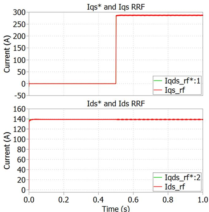
**Figure 11:** The current command (green) and response (red) for a step response commanded torque.
